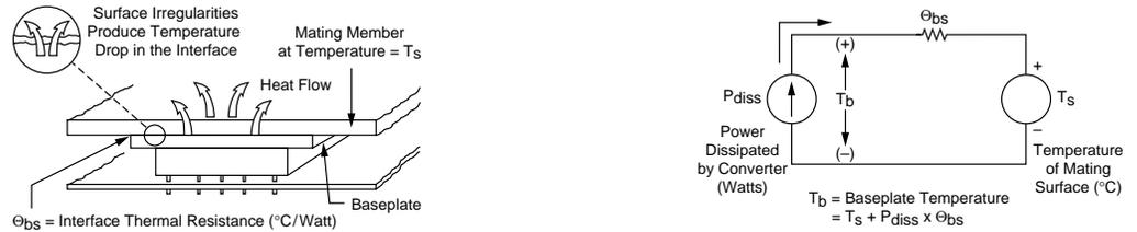
Temperature rise across a surface interface can be significant if not controlled. The area of the interface should be as large as possible, and the surface flatness of the attached member should be within 5 mils. Thermal compound or a thermal pad should be used to fill surface irregularities. Thermal resistance across surface interfaces can be held to under  $0.1^{\circ}\text{C}/\text{Watt}$  with proper measures.
