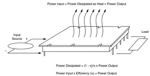
The first step in evaluating cooling requirements is to calculate worst-case dissipation based on converter efficiency and worst-case anticipated load power. Clearly, higher efficiency will translate into lower power dissipation and simplify the cooling problem. Vicor converters are among the most efficient converters available, with full load efficiencies typically in excess of 80%.
